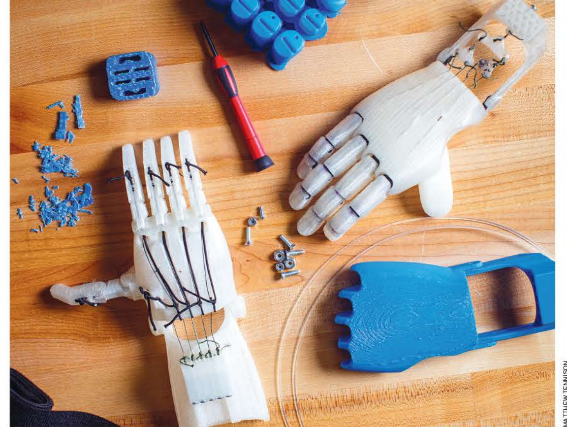
Students downloaded the plans for Raptor Hand, an open-source design online, and adapted it specifically for Emmy.
